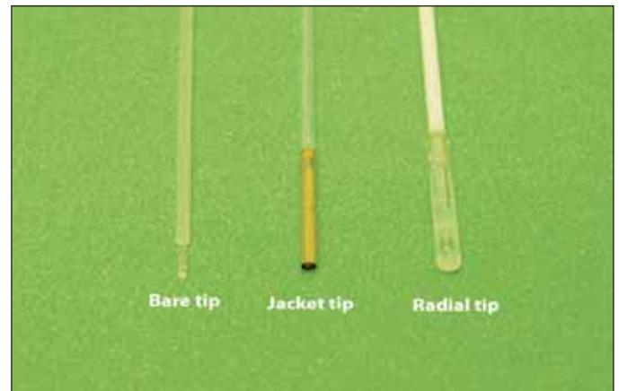
Fig. 3 - Type of Fiber tip.
